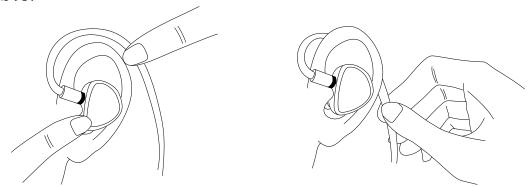
When removing the earphone cable, hold the cable connector and the earphone unit tight with your fingers. Keep them in the same line and then pull them apart. Or use the MMCX assist tool to detach it (Please refer to the instruction of the MMCX assist tool to see how to use it). Note that do not rotate the 0.78mm 2-pin cable.
