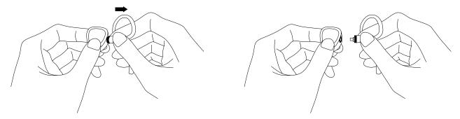
Please do not install or remove the cable at a tilted angle, and do not pull the earphone cable directly, so to avoid it being broken.
