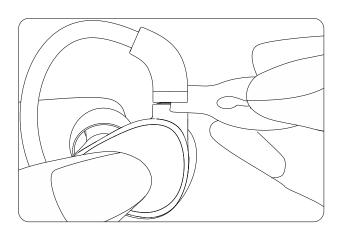
② Ensure the tool is parallel to the gap and position it towards the gap between the connector's male and female components until it is in place.
