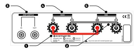
High 4 and mid 5 have separate speaker terminals. In the standard configuration these connectors interconnected with 2 x OFC 2-way bridges 0&9. One bridge 0 interconnects all "+" terminals, the other bridge 2 interconnects all "-" terminals.
