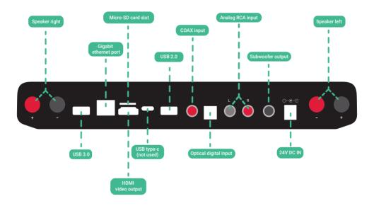
**USB 3.0**: this port can be used to attach USB hi-speed drives, such as SSD, or digital sources such as CD drives.
