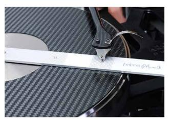
Align the cartridge using the 2 null points on the protractor. The cartridge can be rotated by loosening the cartridge screws. A finer adjustment can be effected by slightly sliding the Sparta mounting board forward or backward.
