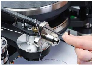
If rotating the counterweight is **not** sufficient to adjust the azimuth, a coarse azimuth adjustment can be effected by loosening the main countershaft screw and rotating slightly the tonearm wand. Retighten the main countershaft screw.
