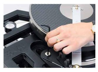
Slide the Sparta armbase so that the mounting cup fits within the circular cut of the protractor. This is a first alignment of the tonearm. It will need to be more precisely ajusted once tje cartridge is installed on the tonearm.
