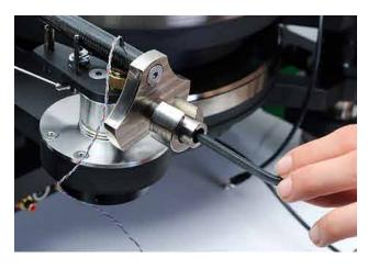
Adjust the azimuth by rotating the counterweight shaft.
