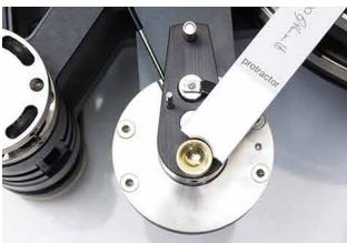
Place the supplied protractor over the platter spindle. Place the other end of the protractor next to the bearing cup.
