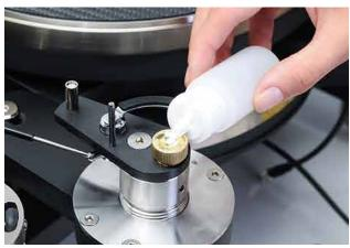
7 Put 2 or 3 drops of the supplied oil in the bearing cup.
