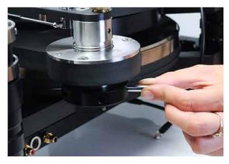
Tighten the delrin nut using the supplied dowel pin.
