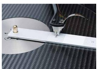
Once the cartridge is properly aligned, fine vta can be adjusted by screwing up or down the bearing cup. A set screw at the back of the base column will lock the base in place.
