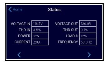
Here you can see the P12's overall performance data. Note how in the above image the THD output is significantly reduced and the output voltage is a stable 120 Volts. Press the Home button to return to the Home screen.
