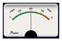
The Power Meter shows the total wattage output from the P12.
