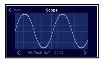
This is a fully functional oscilloscope that you can use to view the incoming AC waveform. Pressing either of the arrow buttons will scroll through the voltage in, voltage out and the difference windows. In this way you can see the degree to which the P12's output waveform is superior to the incoming AC Sine wave.
