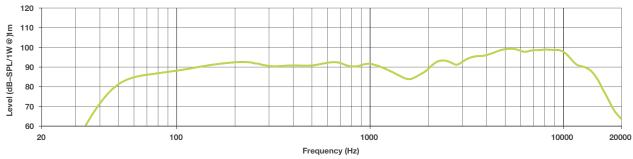
Panaray<sup>®</sup> 802<sup>®</sup> Series IV Installed Sound-Reinforcement Loudspeaker
