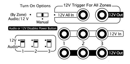
The setting of the rear panel Turn On Options Switch determines whether all three zones turn on and off together or if each zone turns on and off individually. There are three positions for this switch:
