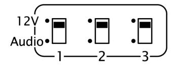
When the Turn On Options switch is set to "Audio/12V By Zone" you can then set the three small 12V/Audio switches to select Audio or 12V turn on/off for each zone. For a zone that you wish to turn on and off by a 12 volt trigger, set that zone's switch to the up position labeled "12V." For a zone you wish to turn on and off by an audio trigger, set that zone's switch to the down position labeled "Audio."
