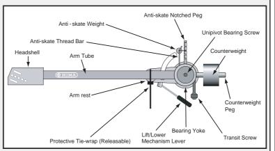
The arm pillar holder fits into a hole 22-23mm diameter and 222-223mm away from the record centre.
