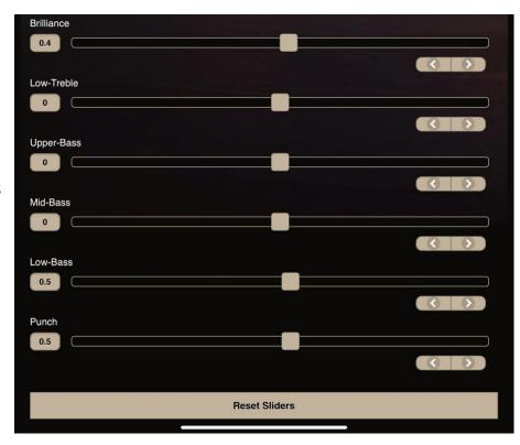
Most speakers benefit from a boost of about +2.5 dB in the brilliance, a low-bass setting of +2 dB with the punch slider set at +2.5 dB.
