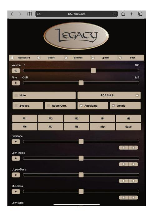
Apodizing allows you to choose between and Apodizing and Linear DAC modes. The Wavelet features an apodizing circuit that corrects for the pre-ringing native to CODECs. Analog lovers can take advantage of balanced XLR or unbalanced RCA inputs without concern of digital artifacts. Turn on the apodization circuit by choosing "Apodizing". When unchecked, the DAC is in linear mode, and the apodization circuit is bypassed. We recommend the Apodizing mode.
