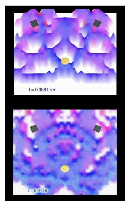
After less than 1/100th of a second, the room has developed a complex wave pattern with energy varying with room position. The listener is now awash in a series of wave-fronts which will soon reflect off the wall behind.
