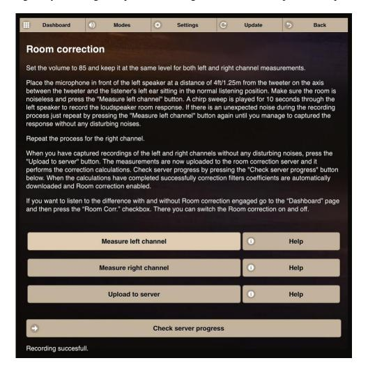
After measuring the left channel, Recording successful will display at the bottom of the screen. If you see an error such as "Volume too low," please check the connections and/or increase the level and measure the left channel again. A successful left channel measurement will display "Recording successful." at the bottom of the screen, as shown above.
