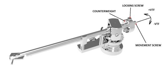
Before setting the Vertical Tracking Force (VTF), confirm the exact weight of your cartridge. Depending on your cartridge weight, determine whether to use the counterweight with or without the additional insert, in accordance with the specifications above.
