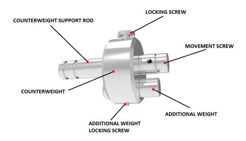
The first part is the counterweight itself. The second part is an additional insert that enables optimal balancing of heavier cartridges.
