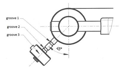
Adjust the anti-skating force by positioning the weight on the appropriate groove of the anti-skating sliding mechanism. Anti-skating down force should be adjusted in correspondence with the tonearm down force as follows:
