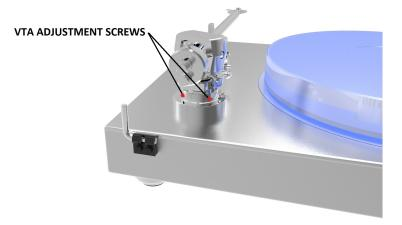
To set the **Vertical Tracking Angle (VTA)**, first put a record (VTF) on the platter. When the needle is lowered into the record groove, the tube of the tonearm should be parallel to the surface of the record. If it is not, loosen both hexagonal screws in the tonearm base, just enough to allow vertical movement of the arm pillar without force, and slide the arm up or down until it is parallel.
