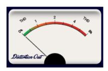
The Distortion Out is a measure of the THD (Total Harmonic Distortion) present in your AC output voltage.
