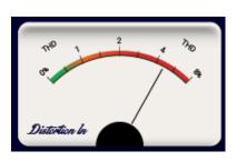
The Distortion In is a measure of the THD (Total Harmonic Distortion) present in your AC input voltage.
