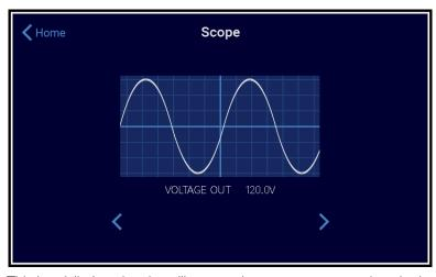
This is a fully functional oscilloscope that you can use to view the incoming AC waveform. Pressing either of the arrow buttons will scroll through the voltage in, voltage out and the difference windows. In this way you can see the degree to which the P15's output waveform is superior to the incoming AC sine wave.
