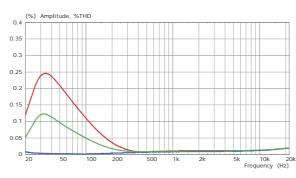
Figure 54. Measured component percentage THD at 20V input level for three capacitors of the same capacitance, but different constructions and manufacturers.
