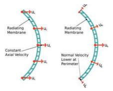
Figure 68. Comparison of tweeter dome axial and surface normal velocity.
