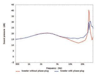
Figure 70. Simulated 1m axis pressure response of thetweeter when driven with a constant unit harmonic acceleration with and without Tangerine waveguide.
