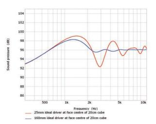
Figure 9. Comparison of the diffraction effect with radiators of different size placed in the centre of a cubic enclosure
