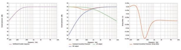
Figure 58. Raw tweeter response (left), 1st order Butterworth crossover using this tweeter (centre), overall group delay (right).
