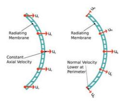
Figure 40. Comparison of tweeter dome axial and surface normal velocity.
