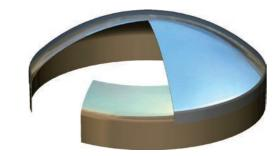
Figure 73. 3D CAD sectional views of the tweeter dome and extended former that meet to form a triangular stiffening member at the dome edge. This patented technology is the KEF stiffened dome.
