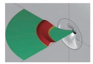
Figure 71. Comparison of a HF transient radiated by a conventional 25mm dome on baffle (left) and an optimally shaped 25mm dome in a waveguide (right).
