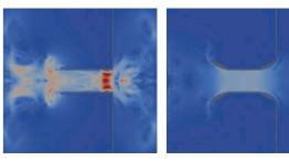
Figure 23. Instantaneous flow pressure contour of straight tube port (left) compared to optimised port (right) computed using CFD, note that both ports are shown on the same colour scale and at the same instant. For this analysis the beak velocity is 10ms.
