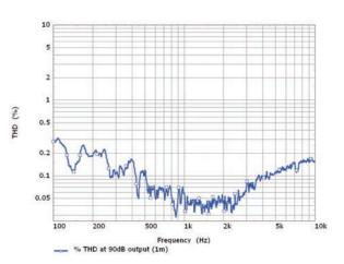
Figure 52. Measured THD of Reference 5 prototype as a percentage of the output SPL at a level of 90dB/1m.
