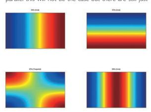
Figure 32. First four standing waves of a rectangular enclosure (left) compared to a trapezoidal enclosure (right)
