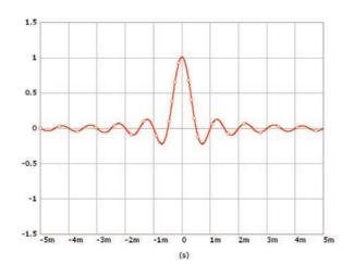
Figure 60. Example of a linear phase filter impulse response.
