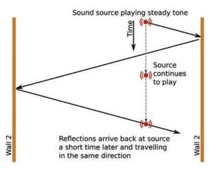
Figure 30. Illustration of standing wave resonance mechanism.
