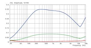
Figure 53. Measured component percentage THD at 20V input level for three inductors of the same inductance, similar cost and similar resistance but different constructions and manufacturers.
