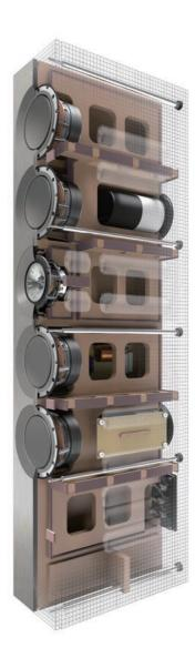
Figure 37. CAD section of Reference 5 showing extensive internal damped bracing.
