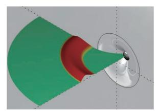
Figure 39. Comparison of a HF transient radiated by a conventional 25mm dome on baffle (left) and a optimally shaped 25mm dome in a waveguide (right).
