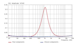
Figure 55. Distortion measurement of full HF crossover at 20V input level with two different component selections, note the component values and filter responses are identical.
