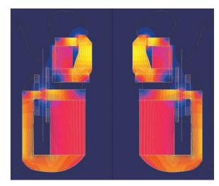
Figure 49. FEA magnetic analysis of Uni-Q motor showing flux density due to bermanent magnets.
