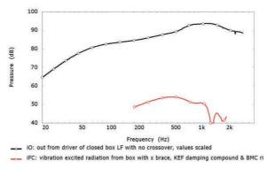
Figure 36. Closed box FEA predicted output from diaphragm and walls with constrained layer of damping material between brace and walls.
