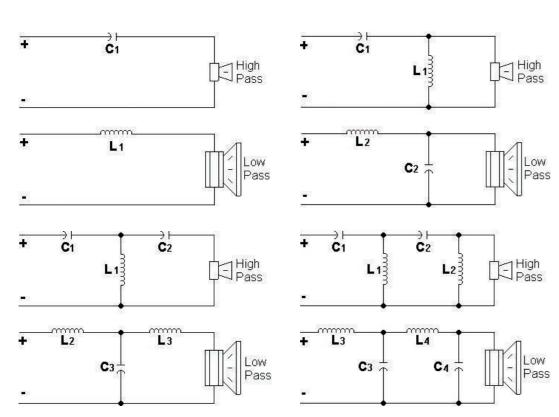
Figure 61. Passive crossover component layouts for 1st (top left), 2nd (top right), 3rd (bottom left) and 4th (bottom right) orders
