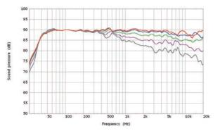
Figure 66. On and off-axis response curves of a well designed Uni-Q system.
