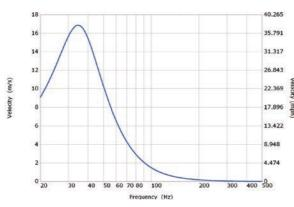
Figure 22. Peak port air velocity for a theoretical 15L speaker at an input level of 10V rms (approx 25Watts).
