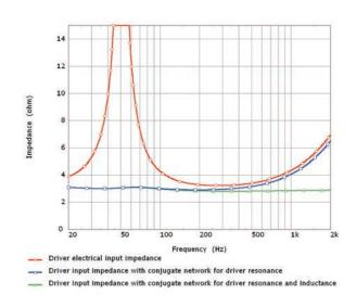
Figure 63. Typical loudspeaker driver electrical input impedance with impedance conjugation components
