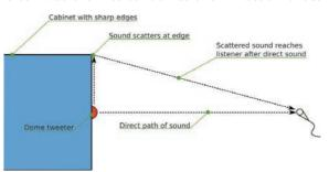
Figure 7. Diagrammatic explanation of diffraction effect.
