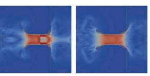
Figure 24. Instantaneous flow pressure contour of unoptimised port (left) compared to optimised port (right) computed using CFD, note that both ports are shown on the same colour scale and at the same instant. For this analysis the beak velocity is 15ms.
