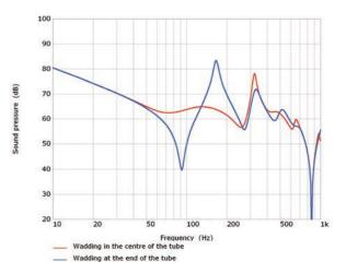
$\textit{Figure 33.} \ \ \textit{The effect of wadding placement on the attenuation of standing waves.}$
