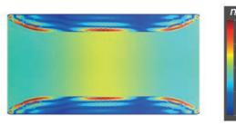
Figure 28. Comparison of the FEA modelled pressure magnitude in the loudspeaker port at the first standing wave with rigid walls (above) and flexible walls (below).
