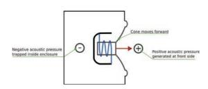
Figure 14. Illustration of a closed box loudspeaker.
