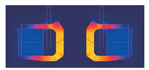
Figure 48. Static magnetic FEA simulation of LF driver motor with flux density shown as colour.
