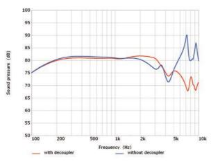
Figure 45. Midrange driver response with and without cone neck control technology.
