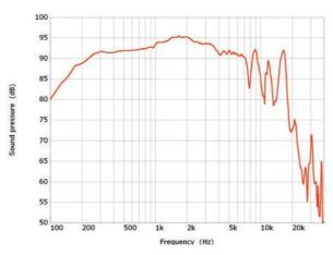
Figure 46. Axial frequency response of the midrange driver measured in 2pi at 1v/1m.
