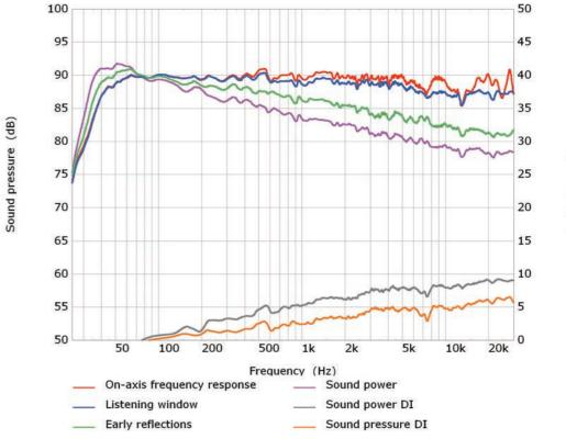
Figure 12. Family of directional response curves for early Reference 5 prototype.
