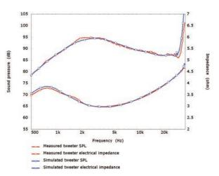
Figure 43. Frequency response of a prototype of The Reference tweeter measured in a test waveguide
