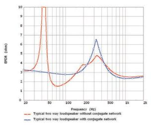
Figure 64. a. Typical closed-box two-way loudspeaker system electrical input impedance with and without a conjugate network in the crossover (left). b. Equivalent Peak Dissipation Resistance for the same two systems (right).
