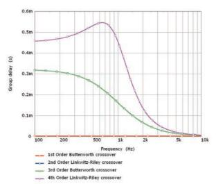
Figure 57. Group delay of classical crossover filter arrangements. Note that the group delay of the 2<sup>nd</sup> order Linkwitz-Riley and the 3<sup>nd</sup> order Butterworth crossover are identical
