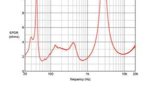
Figure 65. EPDR of Reference 5 prototype system (left) compared to competitor loudspeaker
