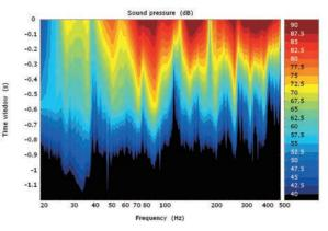
Figure 77. In-room loudspeaker response shown as frequency response chart (left) and short time Fourier response (right).
