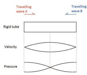
Figure 31. First standing wave pattern (or mode shape) between two parallel rigid
