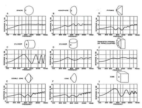
Figure 8. Reproduction of Olsen's classic loudspeaker enclosure baffle-diffraction experiment.
