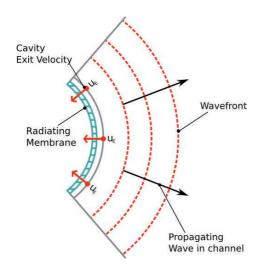
Figure 41. Illustration of the target behaviour of the tangerine waveguide.
