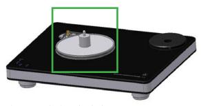
Pic. 7.1: Placing the belt
