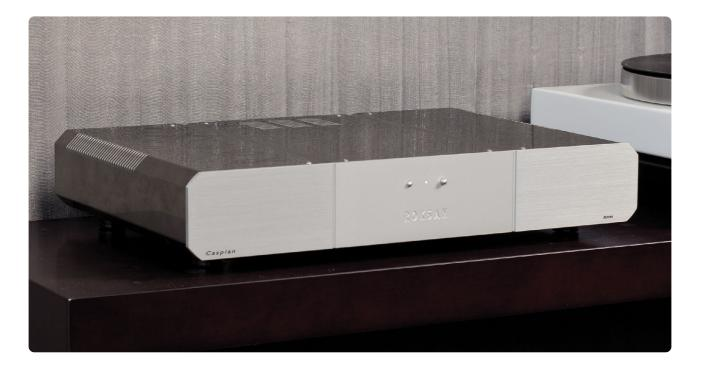
Featuring a super high-quality crystal speed control system and a DS1.5 power supply, it maintains pitch perfect speed stability for both 33 and 45 RPM. It is an upgrade in sound quality and accuracy over XPS 7 (see page 19).
