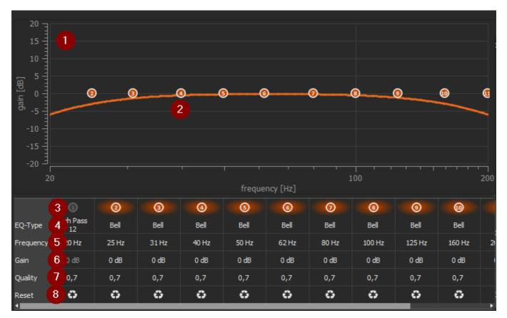
Frequency Response Plot Displays the overall frequency response of the EQs (white line). The EQ handles are located at the center frequencies of the corresponding EQs. The frequency response of a single highlighted EQ is displayed shaded.
