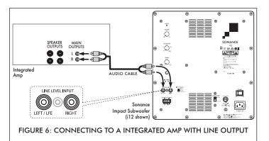
Use a stereo audio cable to connect the integrated amplifier's left and right Line Outputs to the subwoofer's left and right LINE INPUT jacks. If you are installing two subwoofers in the system, connect the integrated amp's left Line Output to the first subwoofer's left LINE INPUT jack and connect the integrated amp's right Line Output to the second subwoofer's right LINE INPUT jack.
