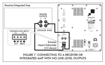
Use speaker wire to connect the receiver/ integrated amplifier's left and right speaker outputs to the subwoofer's left and right SPEAKER INPUTS.
