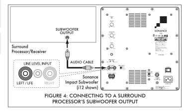
Connect the processor's dedicated Subwoofer Output to the Left LINE LEVEL INPUT jack labeled LEFT/LFE. If you are installing two subwoofers in the system, use a 'Y' connector to connect both subwoofers to the processor's Subwoofer Output.
