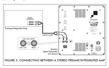
Connect the preamp/integrated amplifier's left and right Main Outputs to the both of the subwoofer's LINE LEVEL INPUT jacks.
