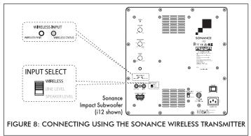
Once your Sonance Wireless Transmitter and your Sonance Subwoofer are powered on, press and release the PAIR button located on the back of the Sonance Wireless Transmitter until the LED light on the front of the unit blinks.
