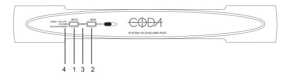
Note: If a power interruption occurs to the system, immediately turn the BIAS power OFF on the front of the SV. The resumption of power will cause no noise pulses in the Amplifier System S150/250. However, some sources may produce high output voltages on turn on, which may cause damage to the amplifier or speakers.
