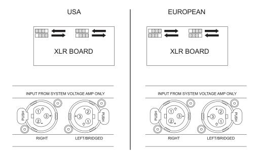
2. The bridging switches are located on the SV main board near the balanced inputs. The default position is STEREO but may be switched to BRIDGED operation according to the following diagram.
