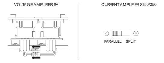
The OPERATION SELECTOR is now commoning both channels of the inputs and both channels of the outputs of the S150/250. The cable from the SV may plug into either LEFT/CH A or RIGHT/CH B input and the speaker leads may be attached to either LEFT/CH A OUTPUT or RIGHT/CH B OUTPUT. The amount of power from each channel is 100 Watts class A (S150), however, since there are two output stages in parallel, current capability is doubled insuring pure class A power into 4 Ohms of 200 Watts .
