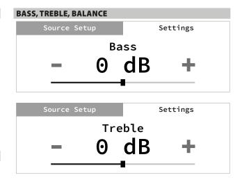
Bass and Treble controls only affect the low bass and high treble leaving the critical midrange frequencies free of coloration.
