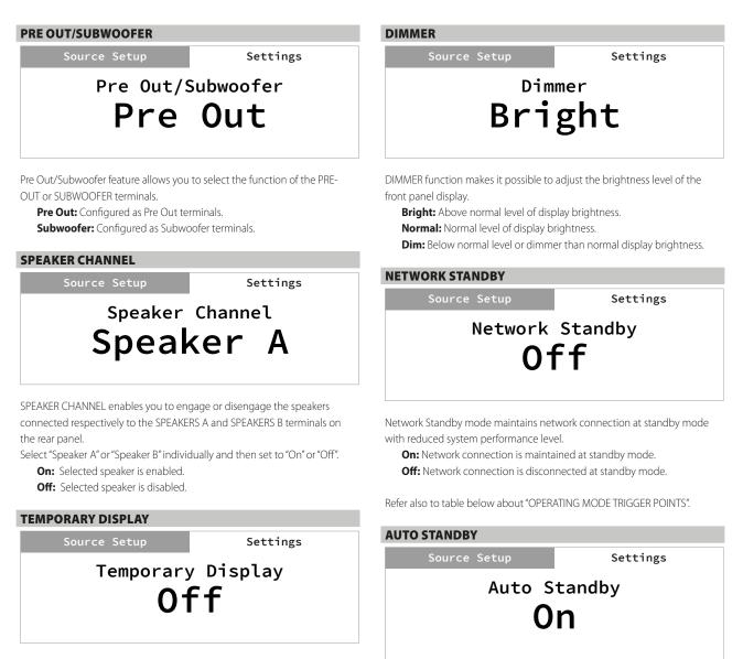
Temporary Display feature enables the display to be turned off temporarily after 10 seconds of non-user interface.
