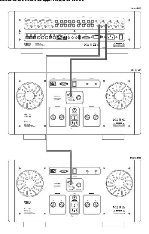
Figure 5-1: 12V Trigger Connections
