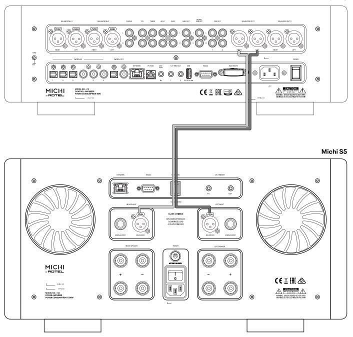
Figure 4-2: Balanced (XLR) Inputs Connection
