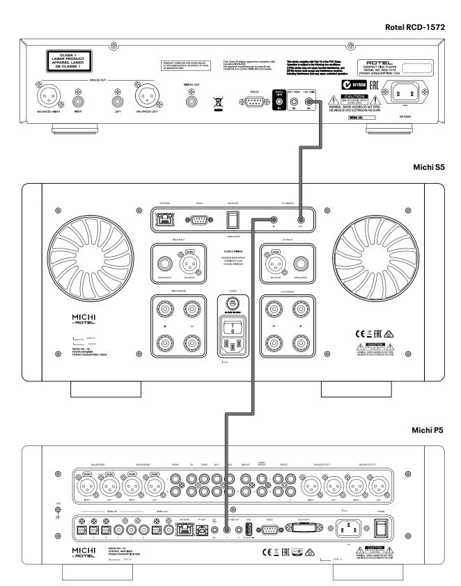
Figure 5-2: 12V Trigger Connections Branchements trigger 12 V 12V-Trigger-Anschlüsse
