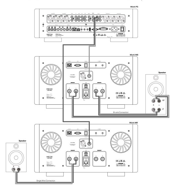
Figure 4-1: Balanced (XLR) Inputs Connection
