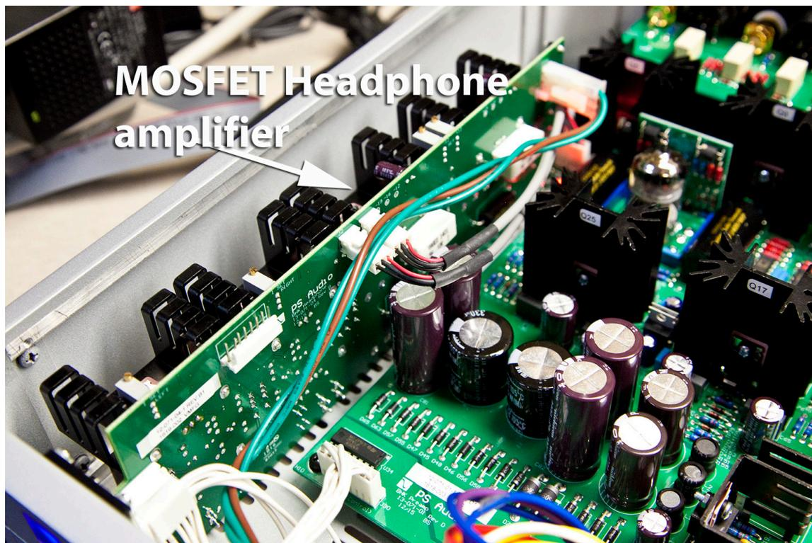
When you insert the headphone jack into the front panel headphone connector, the preamplifier will automatically disconnect the preamplifier outputs. This permits the use of headphones without also having the loudspeakers play at the same time.
