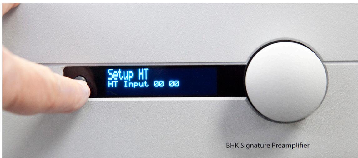
Using the level control, turn the knob until you get to the all zero input. Then press the selector button again to set the choice.
