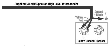
speaker terminal; connect the red wire to the right rear positive speaker terminal, connect the black wire to a ground lug or chassis screw. If the amplifier is of balanced differential design, please follow the instructions in the section above labeled Differential Connection.
