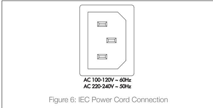
Figure 6: IEC Power Cord Connection
