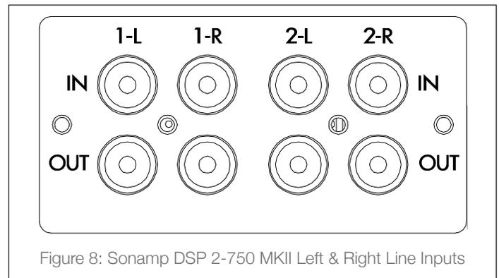
Figure 8: Sonamp DSP 2-750 MKII Left & Right Line Inputs
