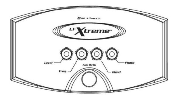
Level: This will allow you to adjust the output volume of the subwoofer. It only controls the subwoofer level, not the level of any of the other loudspeakers in the system, even if they're hooked up in parallel. When using the LFE input, the level can be controlled from your preamp/processor menu while the subwoofer level control can be left at the 12.
