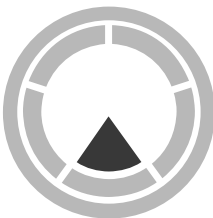
Figure 5.6: Press the sector (or "pizza slice") on the BeoLab 90 interface to change the Beam Width to Narrow.
