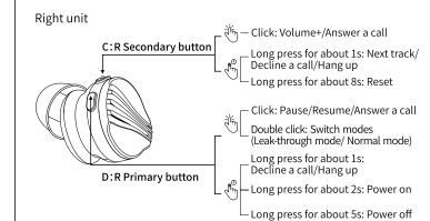
Force into pairing mode: Turn off the FW5. Long press buttons B and D at the same time for about 5s. When the white light of the unit is continuously on for about 3s and then flashes quickly, it will be forced into the pairing mode.
