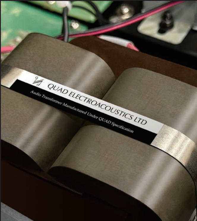
▲ The finest C-Core transformers in the audio path provide excellent linearity, wide bandwidth and very low phase shift.
