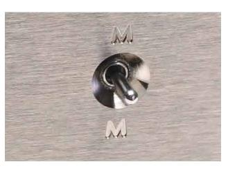
ONCE THE SPEED IS SET: Push the memory switch **up and down** to keep setting in memory. You need to do this for both **33 and 45**. Once set, the system will remain calibrated until a new adjustment is made and memorized. The speed will remain set even if the power supply is disconnected.
