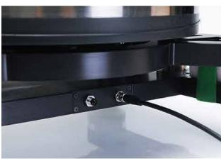
Connect the control cables on the Sparta. There is a 3-pin connector and a 4-pin connector.
