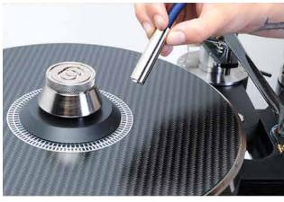
The strobe ca be used to adjust the playback speed. To change the speed, the adjustment toggle switch must be depressed toward the + or -. Each click of the toggle will change the speed in small steps.
