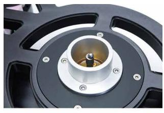
6 Place the bearing ball on the top of the shaft. Make sure the ball stays in place.
