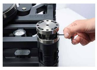
Lock the suspension caps by tightening 2 set screws between the suspension o-rings, as shown.
