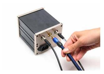
Connect the control cables to the power supply, again being careful to connect the 3-pin and the 4-pin connectors at their rightful location. Connect the strobe cable using the RCA connector.
