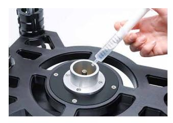
Fill the oil well with 8 ml of Kronos oil. Make sure to put oil on the bearing shaft. Do not use any other oil type. Do not overfill.
