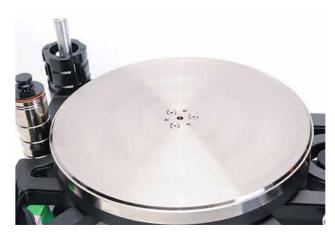
Install carefully the lower platter. Make sure the platter spins freely. If it does not, the ball might have fallen from the top of the shaft. If in doubt, remove platter and start again.
