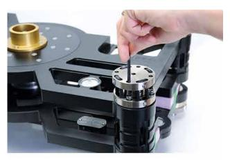
Remove the suspension caps by loosening the screws using the 5/32 spanner.
