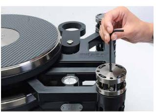
ONCE THE ARM IS IN PLACE: remove the styrofoam spacers. Adjust the top plate level using the adjusters through the center of the suspension caps.
